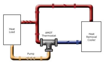
When valves are used for mixing service, Port C is the cold fluid inlet port from the cooler, Port B is the hot by-pass fluid inlet, and Port A the common outlet. Port A is the temperature sensing port and will mix the hot and cold fluids in the correct proportion to produce the desired outlet temperature leaving Port A.
