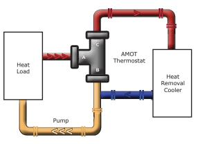
When valves are used for diverting services, the inlet is Port A (temperature sensing port), with Port C being connected to the cooler, and Port B connected to the cooler by-pass line.
